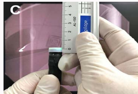
Figure 3C: A 1.5 SIC is fitted to a colonoscope. A ruler measures 1.5mm interval.
