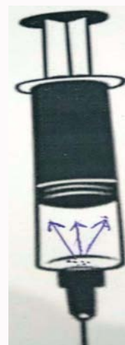
Figure 1: Material is sucked in syringe body and lost.
