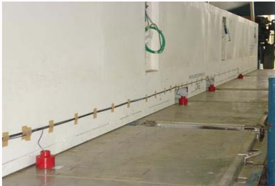
Figure 2: Position of sensors along the pallet.
