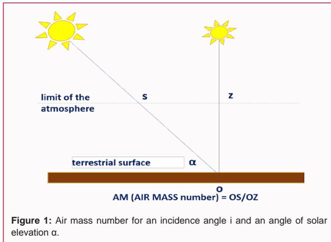
Figure 1: Air mass number for an incidence angle  $i$  and an angle of solar elevation  $\alpha$ .
