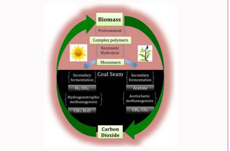
Figure 1: Schematic depicting the concept of low carbon renewable natural gas produced using coal beds as geobioreactors and as sinks for carbon capture and storage.
