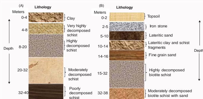
Figure 2: Lithologic section of boreholes in SESB (A) Zuru and (B) Fakai.
