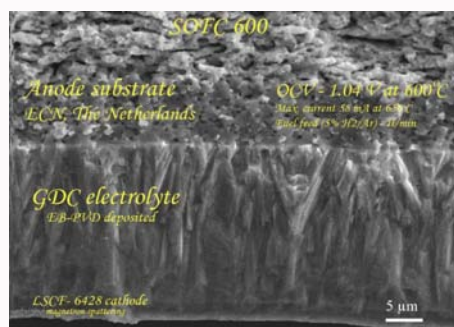
Figure 16: SEM picture of fracture cross-section of CFC made with EB-PVD technique.
