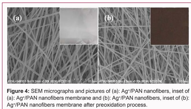
**Figure 4:** SEM micrographs and pictures of (a) Ag<sup>+</sup>/PAN nanofibers, inset of (a) Ag<sup>+</sup>/PAN nanofibers membrane and (b) Ag<sup>+</sup>/PAN nanofibers, inset of (b) Ag<sup>+</sup>/PAN nanofibers membrane after preoxidation process.
