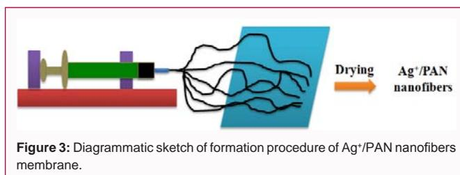
**Figure 3:** Diagrammatic sketch of formation procedure of Ag<sup>+</sup>/PAN nanofibers membrane.
