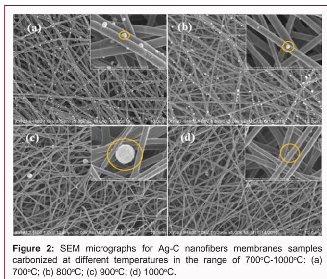
**Figure 2:** SEM micrographs for Ag-C nanofibers membranes samples carbonized at different temperatures in the range of 700°C-1000°C: (a) 700°C; (b) 800°C; (c) 900°C; (d) 1000°C.
