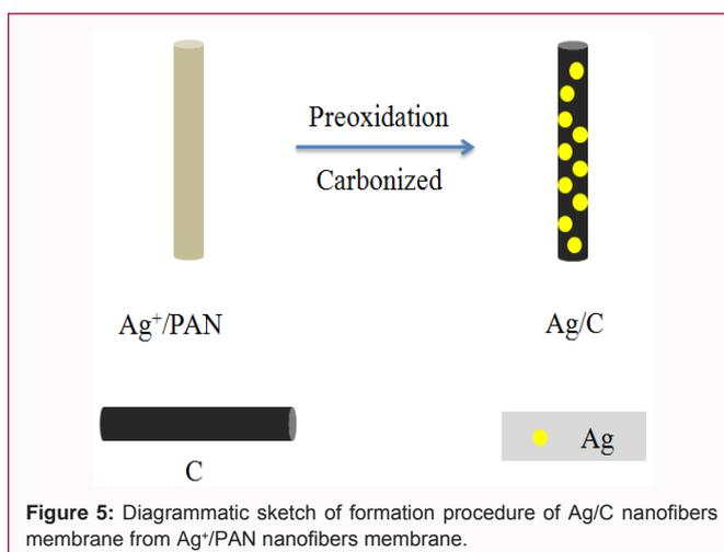
**Figure 5:** Diagrammatic sketch of formation procedure of Ag/C nanofibers membrane from Ag<sup>+</sup>/PAN nanofibers membrane.
